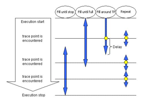
Figure 5.49 Differences between the trace modes
